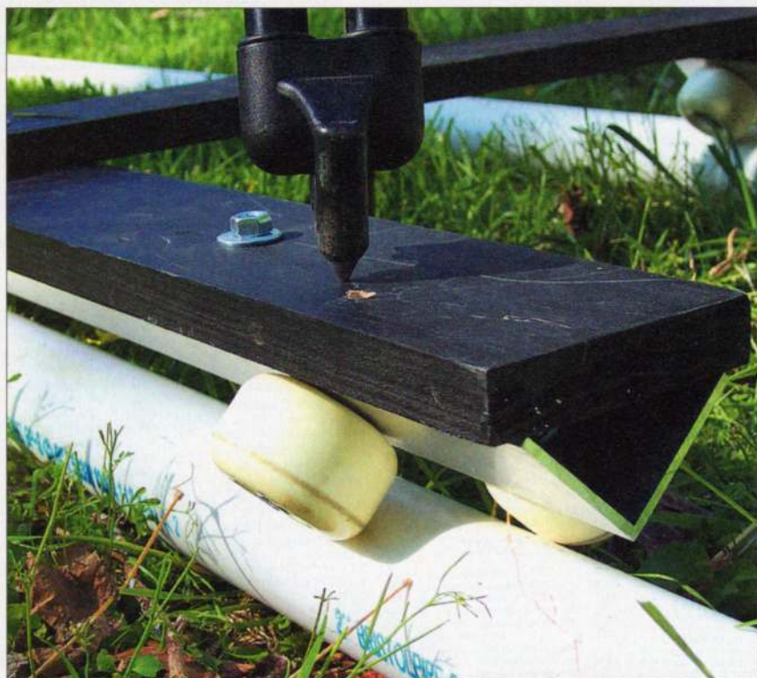
The key component of many low-cost dollies are skateboard wheels bolted at an angle. On Jackman's dolly, an aluminum angle holds the opposing wheels at a 90-degree angle, helping them lock around a 2-inch PVC pipe.
